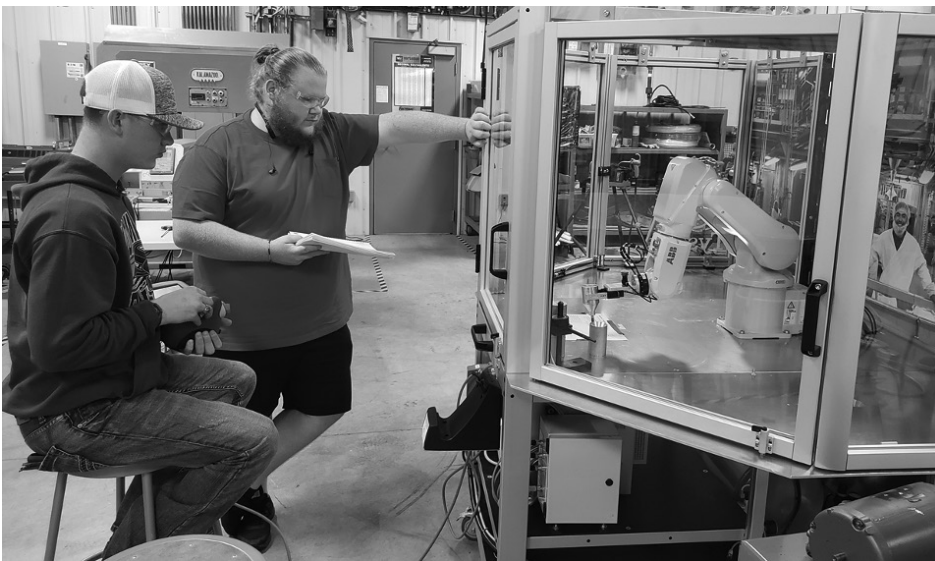
Figure 1. CASS students learning to manually “jog” the IRB 120 industrial robot using the teach pad.
